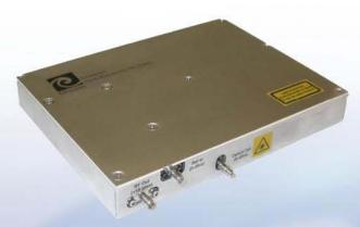
Compact OEO offers extremely *low phase noise* and *low vibration* & acceleration sensitivity for signal source modules required in high-frequency, high performance applications. Available in any output frequency between 10 - 12 GHz (consult factory for other frequencies). Compact OEO offers typical phase noise performance levels of better than - 140 dBc/Hz at 10 KHz offset from the carrier. Compact OEO is offered with a variety of scalable features and options.
