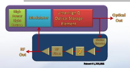
Advanced OEO offers unprecedented *ultra-low close-in phase noise* for signal sources required in high-frequency, high performance applications. Available in any frequency between 8 - 12 GHz (consult factory for other frequencies). Advanced OEO offers typical phase noise performance levels of <u>- 163 dBc/Hz at 10 KHz offset</u> from the carrier. Advanced OEO is offered with a variety of scalable features and options.
